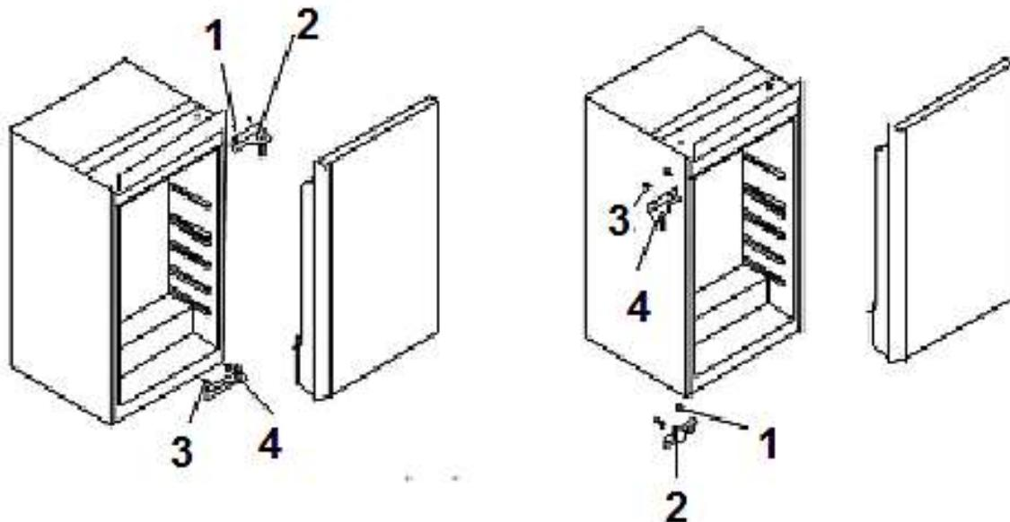
1. Unscrew the 2 screws (1+2) and remove the entire top hinge.
