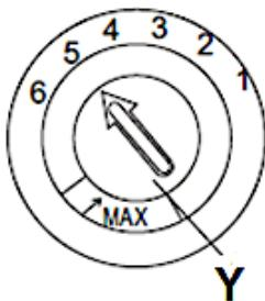
1. Turn the rotary knob to the desired rinse aid consumption level.
