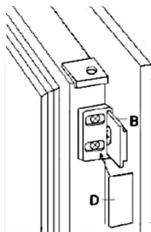
10. Now fix the appliance on the built-in unit. The distance appliance (handle side) to Built-in unit must be 5 mm. The door must close properly. Fix the covers of
