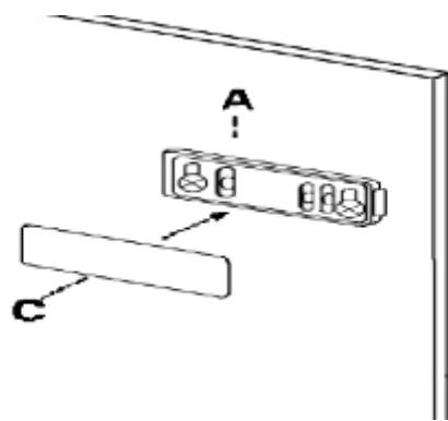
8. Open the doors of the appliance and the built-in unit ( $90^\circ$ ). Insert the small square B in the guide A. Press the doors together and mark the holes (look at figure below). Remove the squares and drill the holes with a diameter of 2 mm in a distance of 8 mm from the outer edge of the built-in unit. Insert square B in the guide A again and fix it with the screws.
