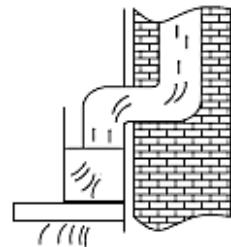
**HORIZONTALLY:** lay the exhaust hose to an exhaust outlet equipped with an air grille\*.
