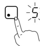
5. Touch the corresponding « BOOST » - SENSOR to activate the « BOOST » - FUNCTION for the selected cooking zone): here in the example the **left** sensor.
