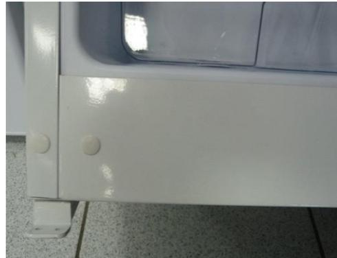
6. Place the door on the bottom hinge. Adjust the door in such a way that it closes properly. Now tighten the screws of the bottom hinge.
