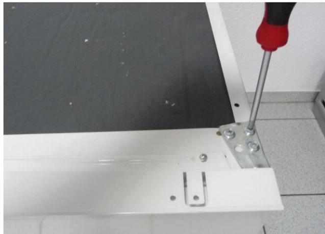
2. Move the top door carefully a bit away from the appliance. Now the door disengages from the hinge. Take the door out of the middle hinge. Keep the door at safe place.
