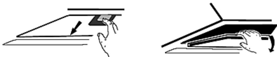
2. The CARBON FILTER is installed on the motor.
