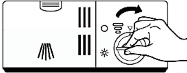
**i** Do not forget to replace and tighten the lid of the rinse aid container **after** filling.
