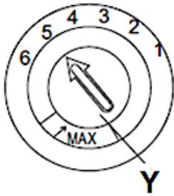
1. Turn the rotary knob to the desired rinse aid consumption level.
