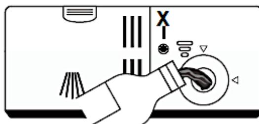
3. Replace the lid (as shown on the figure below) and turn it firmly (in clockwise direction / s. fig. below, arrow direction).
