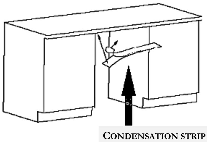
**NOTICE!** Improper installation of the condensation strip may cause damage to the worktop.
