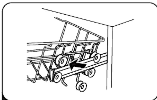
4. Replace the dish rack (**A**), positioning the guide rails (**B**) between the middle (**D**) and the lower wheel sets (**E** / s. fig. below).
