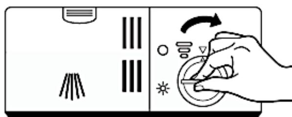
**■** Do not forget to replace and tighten the lid of the rinse aid container **after** filling.
