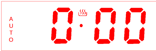
Pic 14 Cooking time setting initial state
