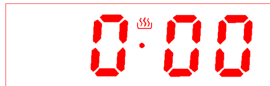
Pic 7 Feature to be selected state diagram (second icon always bright)
