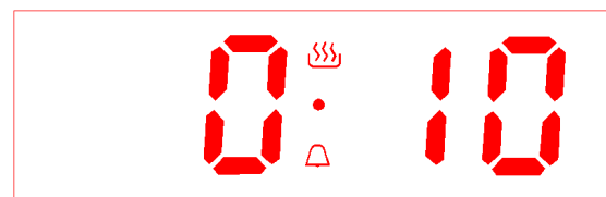
Pic 10 Alarm clock well set (alarm clock icon flickering)
