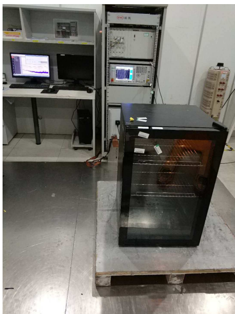
Continuous Disturbance Voltage
