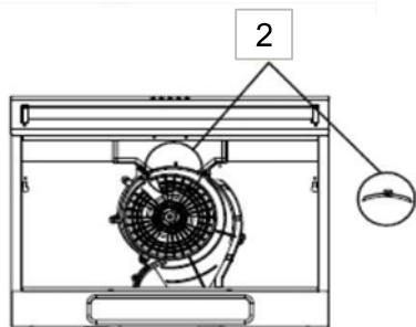
Do not remove the mode selection block (**Fig. 1**) for exhaust air operation.
