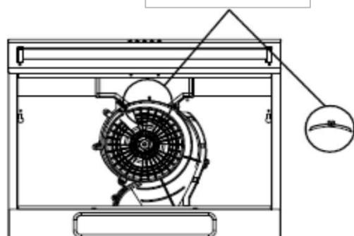
Then mount the carbon filter by guiding it to the filter holder at the bottom of the motor and tightening it by turning it clockwise. (Bayonet lock)
