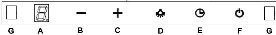
1. After connecting the cooker hood to the socket, the background lighting of all buttons is switched on. The LED display "A" does not light up. The cooker hood has no function and is in standby mode. The backlight of all buttons is automatically switched off after 2 seconds without any operation.
