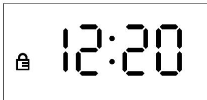
Pic 10: Door lock activated display effect
