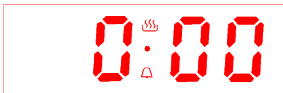
Pic 11 Alarm clock working status diagram Pic 12 Alarm clock time over diagram (alarm clock icon always bright) (alarm clock icon flickering)
