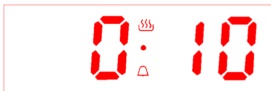
Pic 11 Alarm clock working status diagram Pic 12 Alarm clock time over diagram (alarm clock icon always bright) (alarm clock icon flickering)
