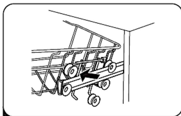
9. Replace the dish rack (**A**), positioning the guide rails (**B**) between the middle (**D**) and the lower wheel sets (**E** / s. fig. below).
