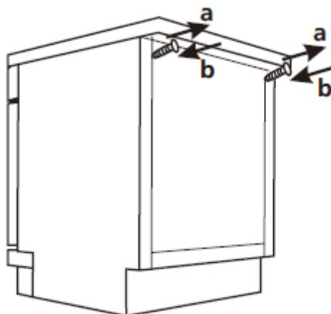
**NOTICE!** After removing the work top, the screws must be screwed again under the rear edge of the top (b).
