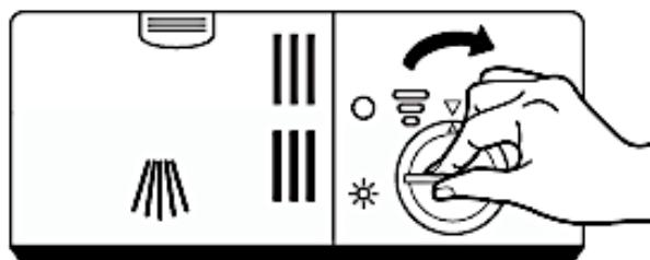
**i** Do not forget to replace and tighten the lid of the rinse aid container **after** filling.
