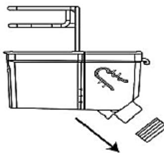
4. Attach the O-sealing ring to the bottom of the water tank. Make sure that there are no folds or creases in the process.
