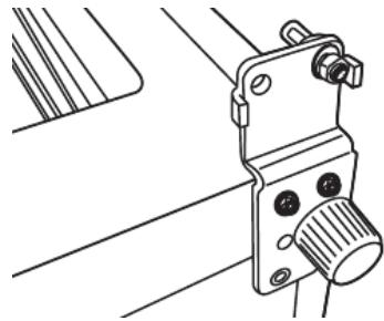
6. Remove the hinge pin (1) and fix it in position 2. Fix the hinge on the opposite side. Fix the foot.
