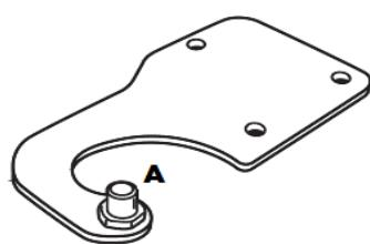
4. Remove the hinge insert plate from the bottom of the door and fix it on the opposite side.
