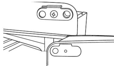
5. Tilt the appliance by max.  $45^{\circ}$  and remove the feet and the screws securing the right hand hinge plate, and the fixing plate.
