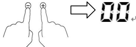
After setting the timer, the decimal point of the single digit display of the burner which is set timer will be light on. And the two digits display will show the minimum timing among all the timers.
