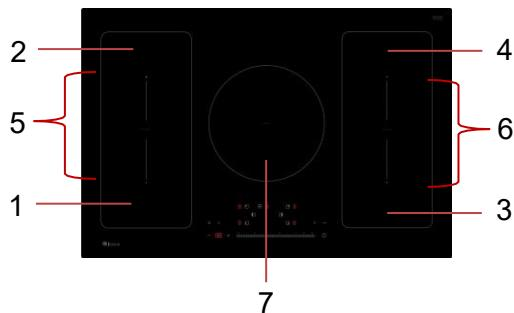
1.  $\Phi 180\text{mm}$  Max:1600/1800W
