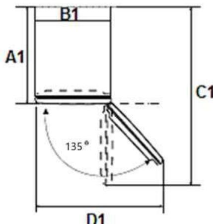
**A 1= Depth / B 1 = Width / C 1 = Depth (when the door is open) /
