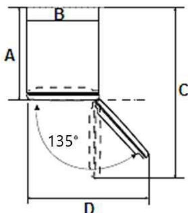
A = Depth / B = Width / C = Depth (when the door is open) /
